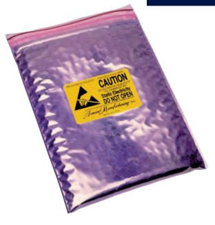
Maximum ESD protection in a three ply pouch with Faraday cage constructions featuring an inner layer of static dissipative .004 poly meets electrical and physical properties of MIL-PRF-81705, Type II, a mid layer of Cancel® cushion meets PPP-C-1842 Type I and CID-A-A-3129 Type I; a static shielding outer meets electrical and physical properties of MIL-PRF-81705 Type III outer layer. Armand's multi-layer construction offers static shielding and impact resistance all in one bag.
