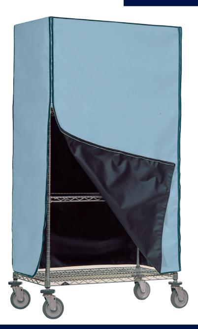
Maximum ESD protection is provided with blue/black dissipative/conductive supported vinyl cart cover. Designed to shield static sensitive devices, components and sub-assemblies from ESD damage, dust and dirt during transportation and storage. Blue side is static dissipative black side is conductive. Covers are washable, durable, flame resistant, mildew / fungal resistant, reusable, form-fitted to the product.
