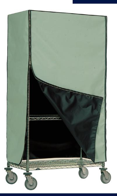
Maximum ESD protection is provided with green/black dissipative/conductive supported vinyl cart cover. Designed to shield static sensitive devices, components and sub-assemblies from ESD damage, dust and dirt during transportation and storage. Green side is static dissipative black side is conductive. Covers are washable, durable, flame resistant, mildew / fungal resistant, reusable, form-fitted to the product.
